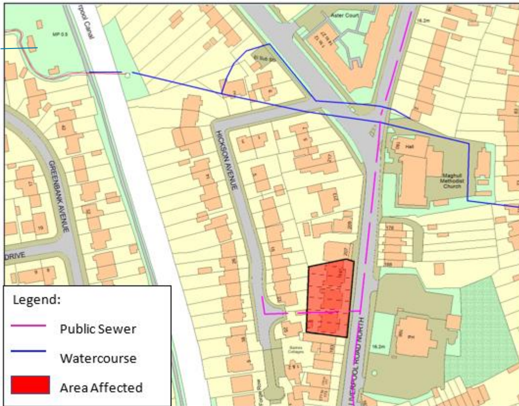
Figure 4 Drainage network 187-197 Liverpool Road North
